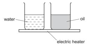
The temperature of the water and the temperature of the oil increase steadily. The increase in temperature of the oil is much greater than that of the water.
